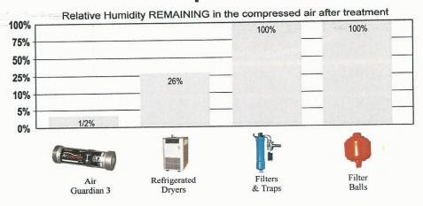
Filters and traps DO NOT REMOVE ANY MOISTURE VAPOR from the compressed air, they simply remove liquid water from the air line.
